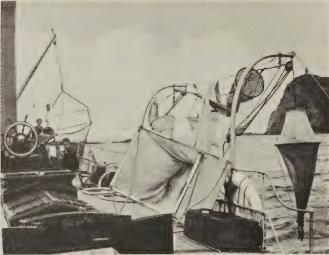
FIG. 6. Some plankton nets, shear-net, &c., on S.Y. "Ladybird." The Agassiz trawl is seen in the distance hanging from the derrick.
